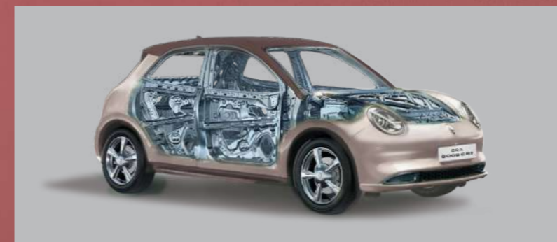
65% High Strength Steel Throughout Vehicle Body
