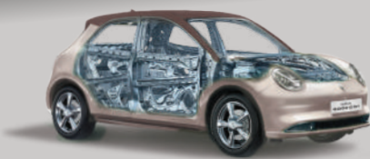
65% High Strength Steel Throughout Vehicle Body
