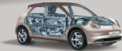
65% High Strength Steel Throughout Vehicle Body
