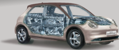
65% High Strength Steel Throughout Vehicle Body
